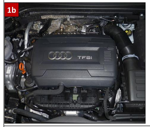
Pull the engine cover carefully upwards
