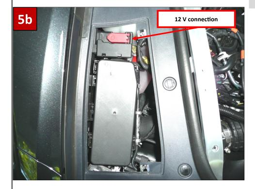
Connect the red cable of the new wiring harness to the positive pole of the battery.
