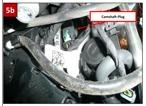
Disconnect the plug from the camshaft sensor.
