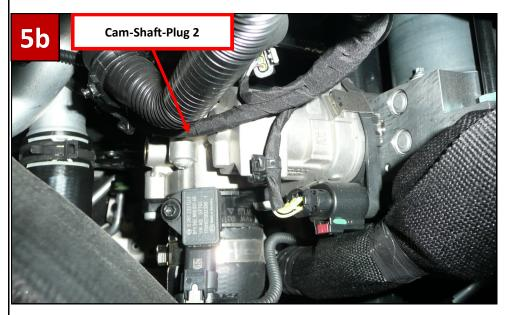
Disconnect the plug from the camshaft sensor.
