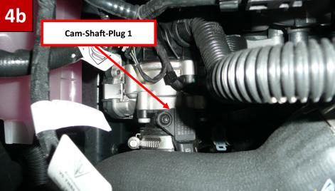
Disconnect the plug from the camshaft sensor.
