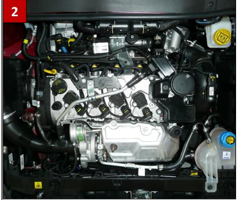
♦ The engine cover is clipped to the engine
